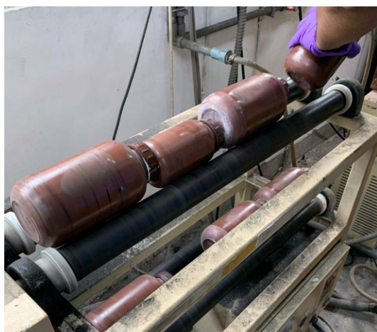
Figure 10: Machine that spins the bottle with mixture
